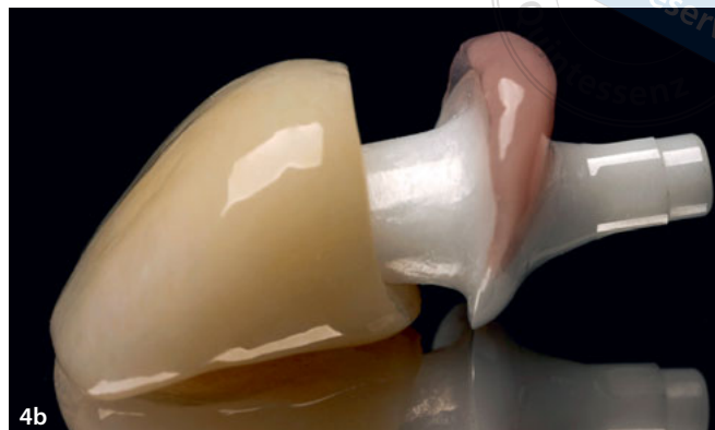
Figs 4a and 4b One-piece all-ceramic implant abutment, second generation, with internal connection (Internal Interface, Bone Level; Straumann). The zirconia abutment, which had been customized from a semi-finished CAD/CAM product, was modified with a gingival mask made of sintered ceramics and then restored with a lithium disilicate ceramic crown (build-up technique, IPS e.max Press; Ivoclar Vivadent). (Laboratory procedures: Oliver Brix, CDT, Bad Homburg, Germany).
